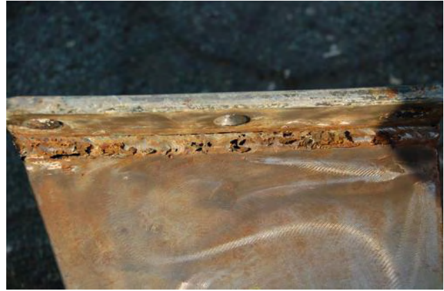
If your sailboat keel is bolted on, check the bolts and the keel itself. This strut was replaced.
